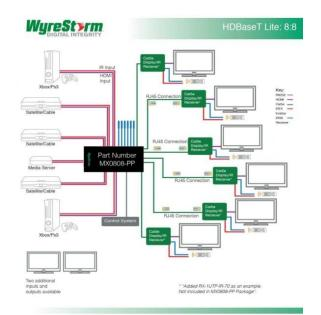
To distribute the 6 satellite boxes throughout, a  $8\times8$  Wyrestorm Matrix was incorporated and everything was communicated using HDMI over Cat6 systems. This gave the yacht flexibility and the ability to upgrade from one central point
